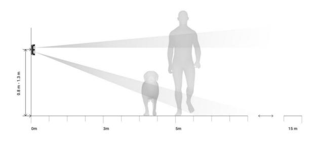
The detector recognizes motion and sends the first alarm immediately, but next alarms until disarming are transmitted no more than once in 5 seconds.
