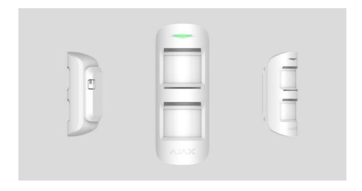
MotionProtect Outdoor is a wireless outdoor motion detector for the Ajax security system. The detector communicates with the hub via protected Jeweller radio protocol at a distance up to 1,700 meters in the line of sight. MotionProtect Outdoor features protection against blocking the detector view (anti-masking system) and triggering by pets (pet immunity). The motion detection distance is adjustable: from 3 up to 15 meters.
