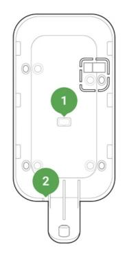
1. A cap for putting out the power supply wire behind the SmartBracket attachment panel
